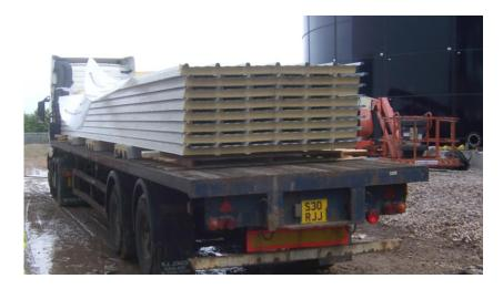
The purpose of the X-dek bearers is to allow un-loading beams to pass through the bearers and the locations of the bearers are agreed with Kingspan to suit the Pack Boy<sup>TM</sup> modular off-loading system. Refer to the separate chart detailing Pack Boy<sup>TM</sup> beam centres, lifting capacities and lift heights for details.
